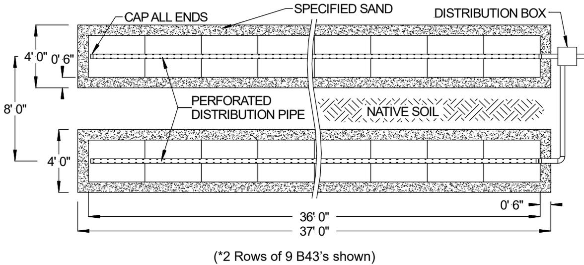
FIGURE 7: SECTION VIEW – TRENCH SYSTEM EXAMPLE – LEVEL SITE
