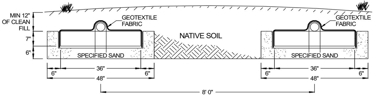
FIGURE 8: SECTION VIEW – TRENCH SYSTEM – SLOPING SITE
