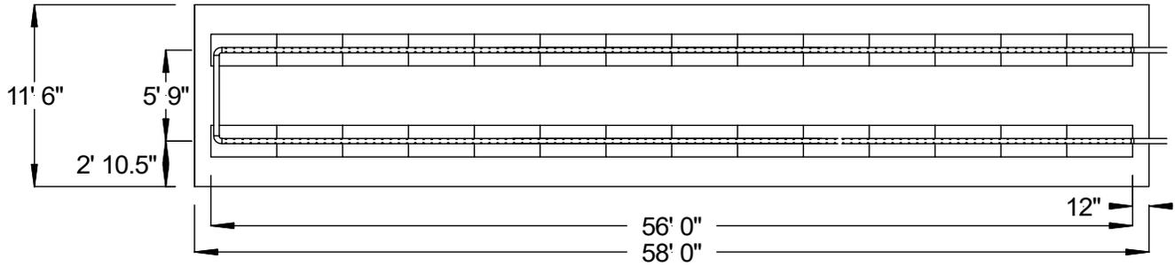
FIGURE 12: SECTION VIEW – BED SYSTEM EXAMPLE
