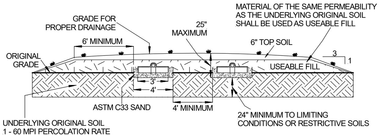
**2.15 SYSTEM GEOMETRY:** Design systems as long and narrow as practical along site contours to minimize ground water mounding especially in poorly drained low permeability soils. If possible, design level systems with equal number of modules per row.
