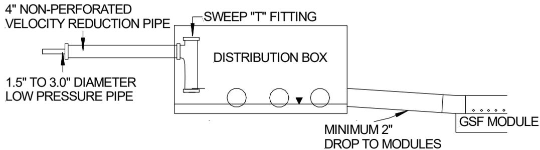
**6.2 DOSING DESIGN AND FLOW RATE:** Set the floats or pump time controls to deliver a maximum of 4 gallons per B43 module for each dosing cycle. Additional volume for the effluent draining back to the dose tank may be added to this volume.
