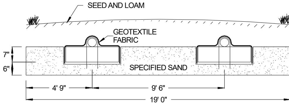
FIGURE 11: SECTION VIEW – SLOPING BED SYSTEM
