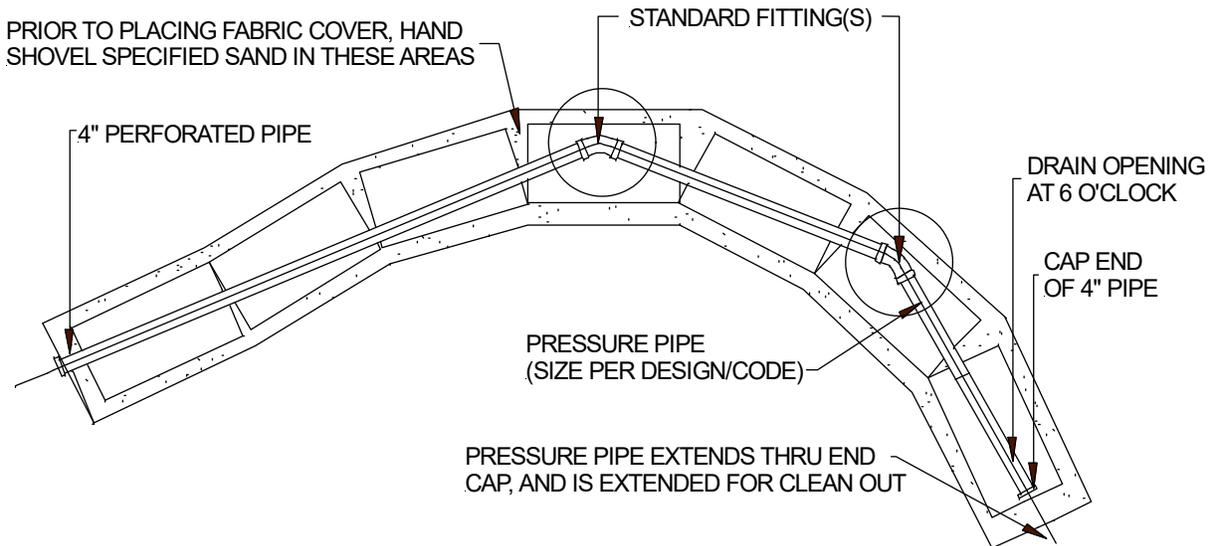
GSF Pressure Distribution trench placed on a contour or winding trenches to maintain horizontal separation distances may also be used in Dosed or Gravity system by removing the pressure pipe and using the 4-inch diameter perforated distribution pipe.
