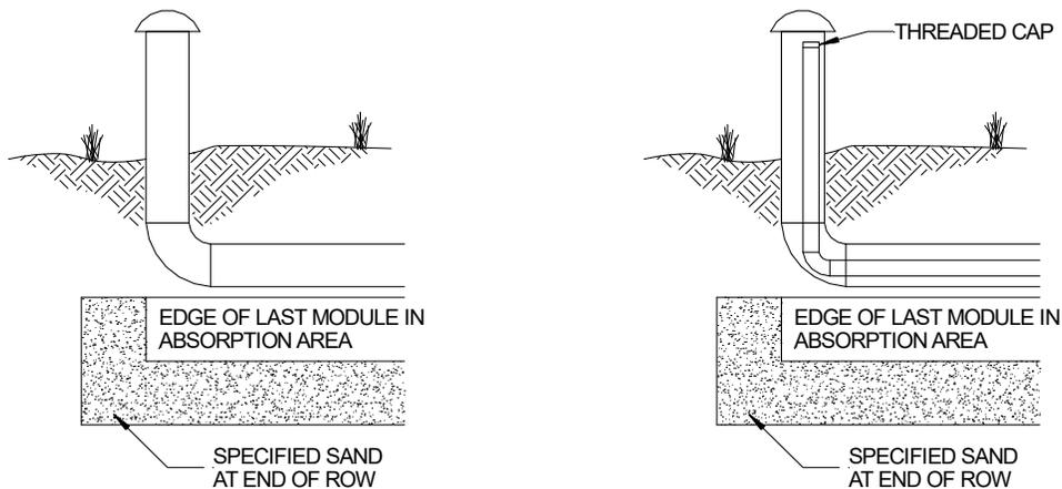
**8.3 AIR BY-PASS LINE:** Systems with over 18" of cover that are pumped or pressure dosed require an air by-pass line to continue flow from the low vent on the system to the high vent of the house. Simply plumb an airline from the distribution system back to the pump chamber or septic tank to provide unobstructed flow.
