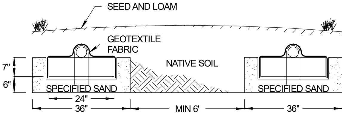
FIGURE 8: SECTION VIEW – TRENCH SYSTEM – SLOPING SITE
