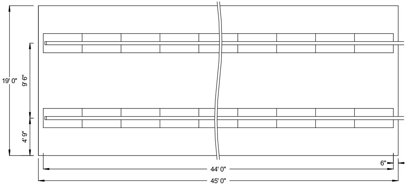
FIGURE 10: SECTION VIEW – BED SYSTEM
