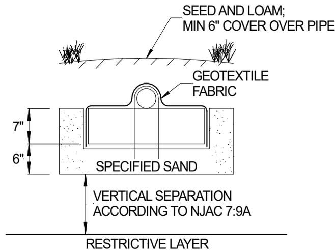
**2.4 SPECIFIED SAND SPECIFICATION FOR GSF SYSTEMS:** The sand immediately under, between rows and around the perimeter of the GSF system must meet ASTM C33 Sand Specification, **WITH LESS THAN 10% PASSING A #100 SIEVE AND LESS THAN 5% PASSING A #200 SIEVE**. Please place a prominent note to this effect on each design drawing. See Table 1 for more information on the sand and sieve specifications.
