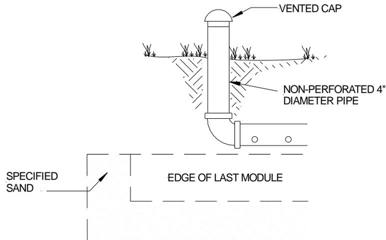
**7.2 VENT PIPE FOR LOW PRESSURE DISTRIBUTION SYSTEMS:** If the system is a low-pressure distribution system with greater than 18 inches of cover, ensure that the LPP clean outs are located in the vent for easy access.
