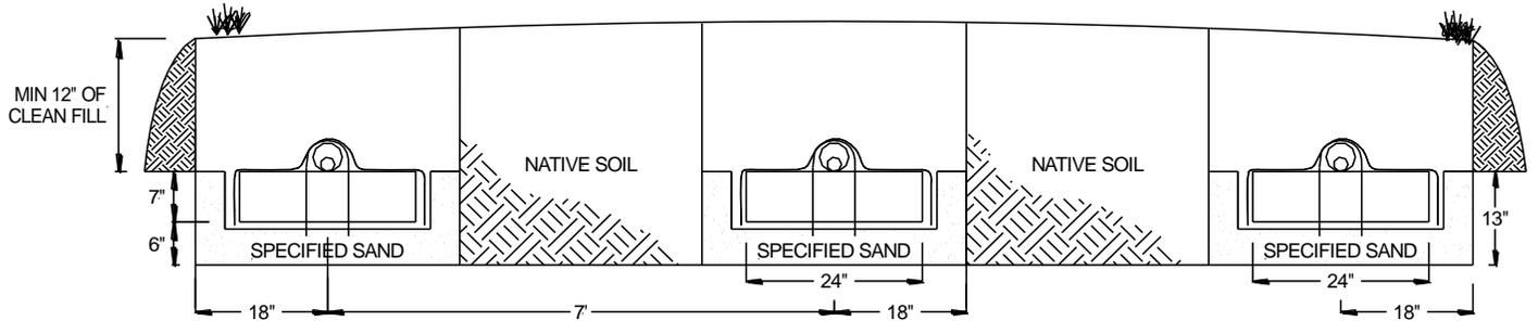
FIGURE 4: SECTION VIEW – A42 TRENCH SYSTEM – SLOPING SITE
