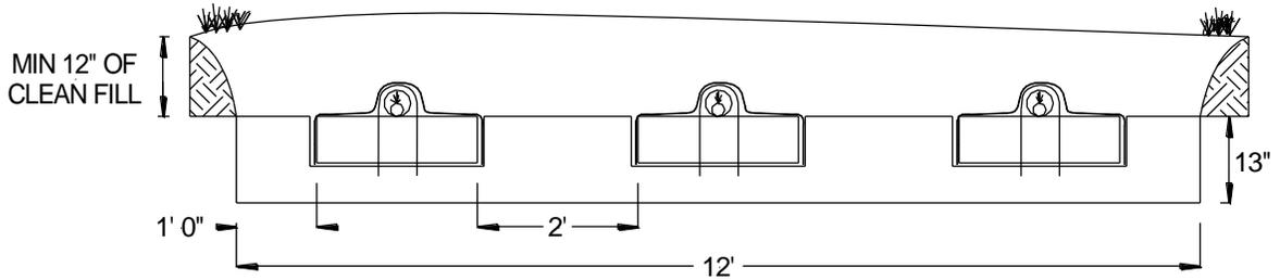
FIGURE 10: SECTION VIEW – A42 BED SYSTEM – SLOPING SITE
