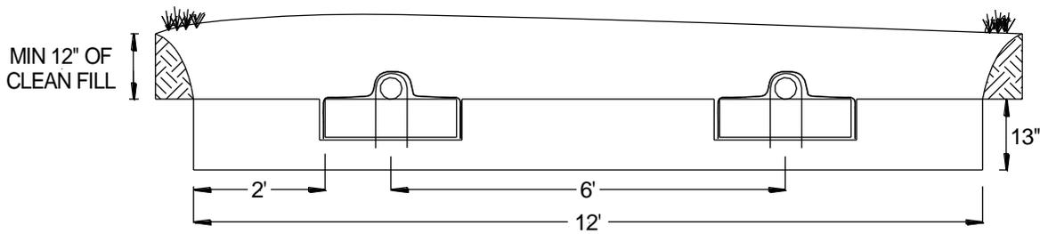
FIGURE 7: SECTION VIEW – A42 BED SYSTEM – SLOPING SITE
