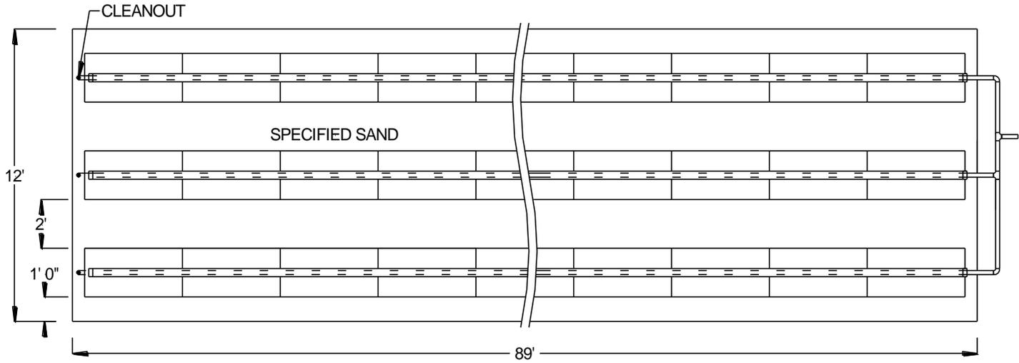
FIGURE 9: SECTION VIEW – A42 BED SYSTEM – LEVEL SITE
