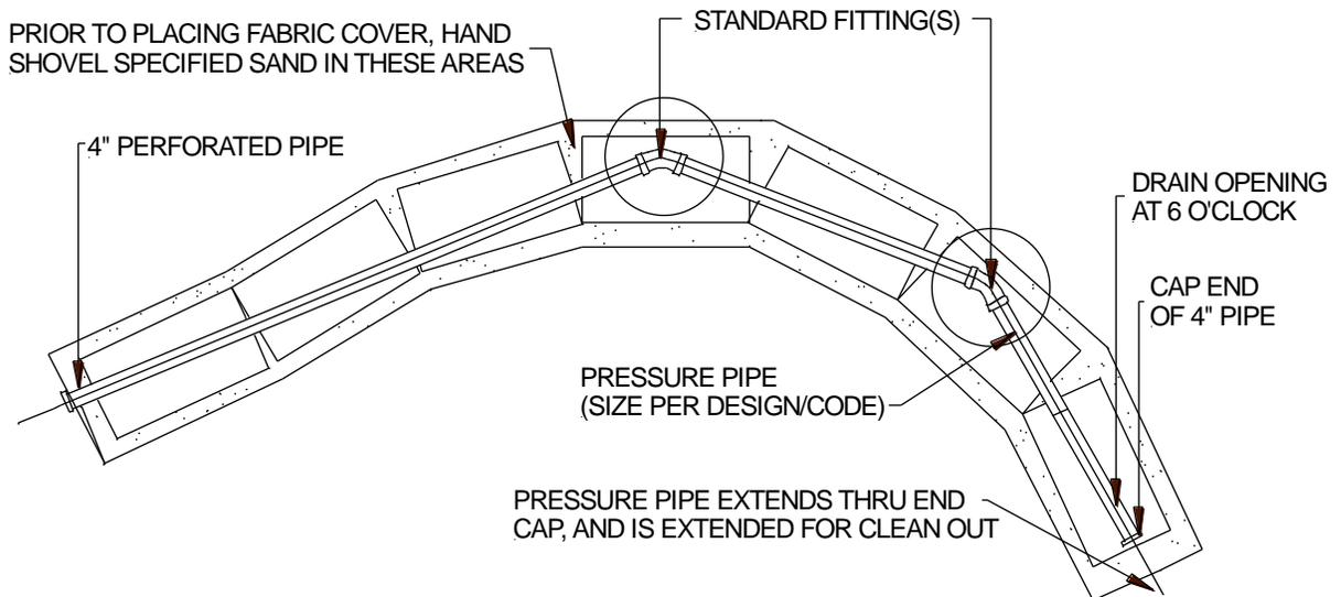
GSF Pressure Distribution trench placed on a contour or winding trenches to maintain horizontal separation distances.
