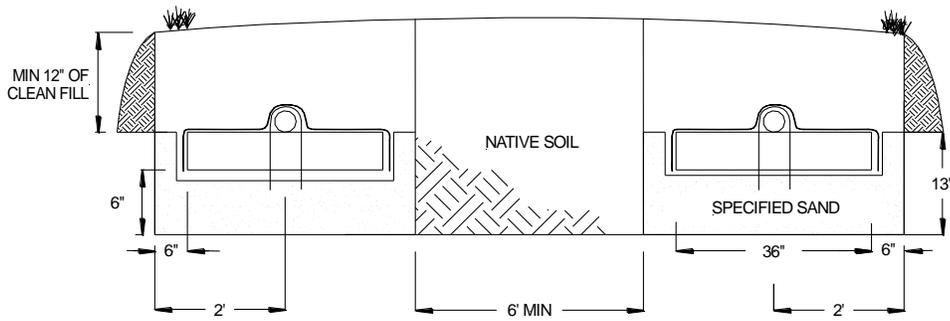
FIGURE 5: SECTION VIEW – 600 GPD – TRENCH SYSTEM – SLOPING SITE
