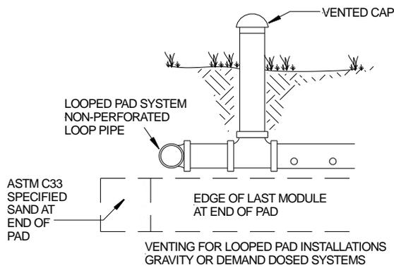
**9.2 VENTILATION FOR PRESSURE AND DEMAND DOSED SYSTEMS:** If a pressure or demand dosed system is specified with greater than 18 inches of cover, an additional 2-inch minimum air line must be extended from the GSF Drop Box back to a knockout or riser on the septic tank or pump chamber. This maintains the continuity of airflow from the field into the house plumbing.
