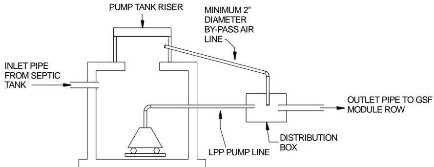
**9.3 VENT PIPE FOR LOW PRESSURE DISTRIBUTION SYSTEMS:** If the system is a low pressure distribution system with greater than 18 inches of cover, ensure that the LPP clean outs are located in the vent for easy access.
