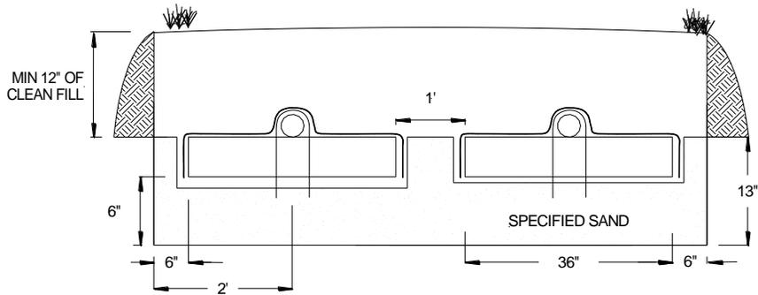
FIGURE 8: SECTION VIEW – 450 GPD – BED SYSTEM – SLOPING SITE
