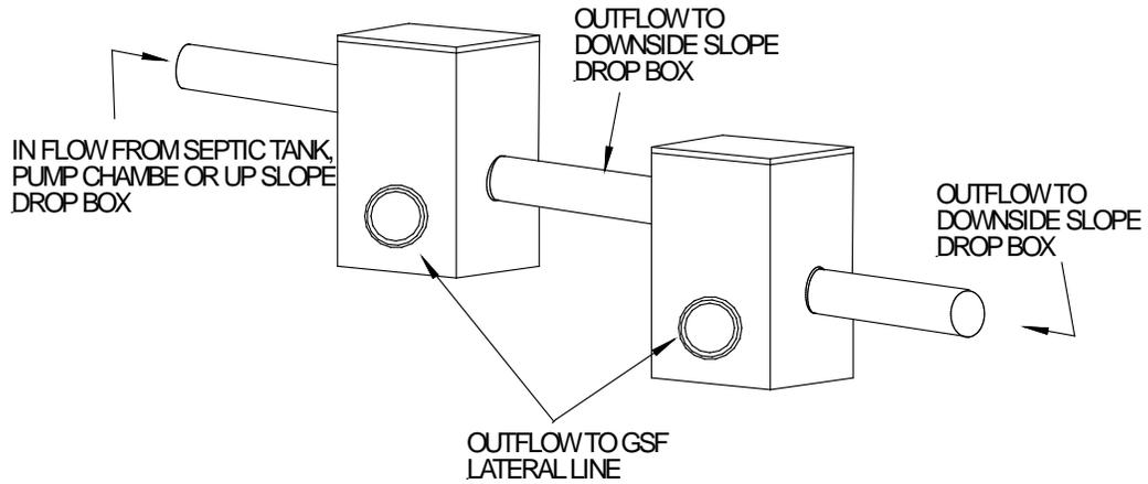
**FIGURE 13: TYPICAL RAISED BED DESIGN**
