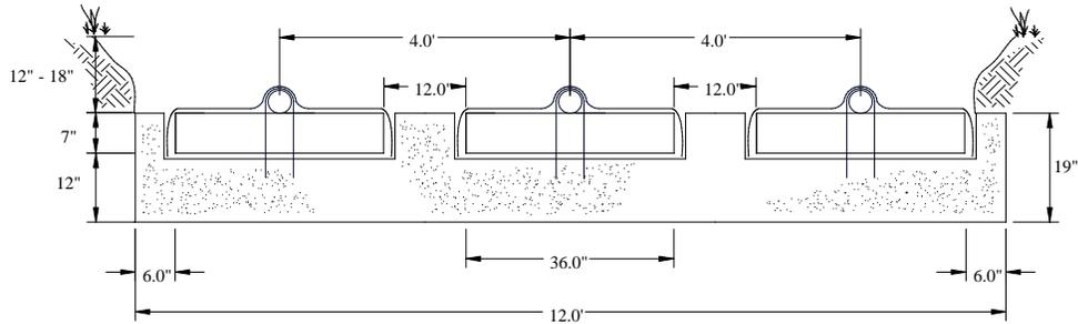
**FIGURE 11: TYPICAL SLOPED B43 BED CROSS SECTION DESIGN**
