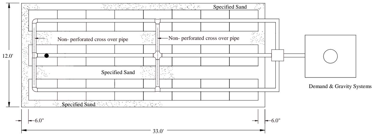
**FIGURE 10: TYPICAL B43 BED CROSS SECTION DESIGN**
