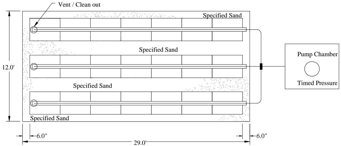
**FIGURE 9: B43 BED DESIGN NON-PERFORATED CROSS OVER PIPES**
