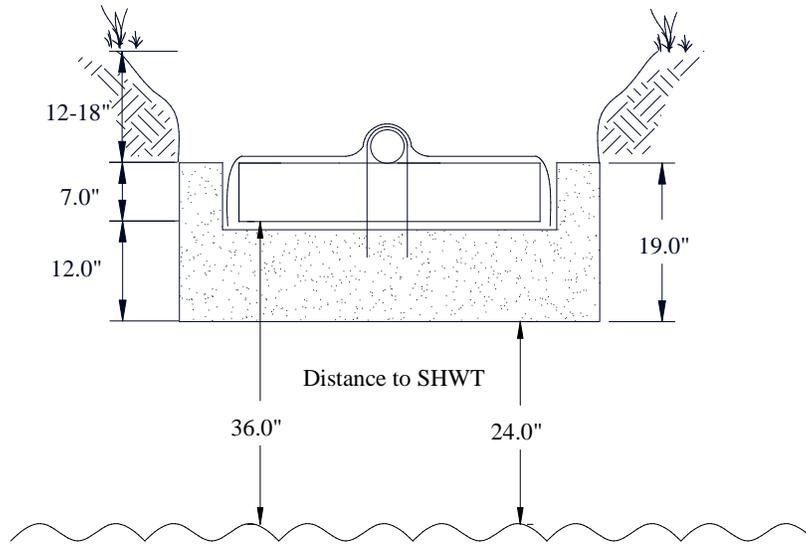
**FIGURE 4: B43 GSF TRENCH CROSS SECTION**
