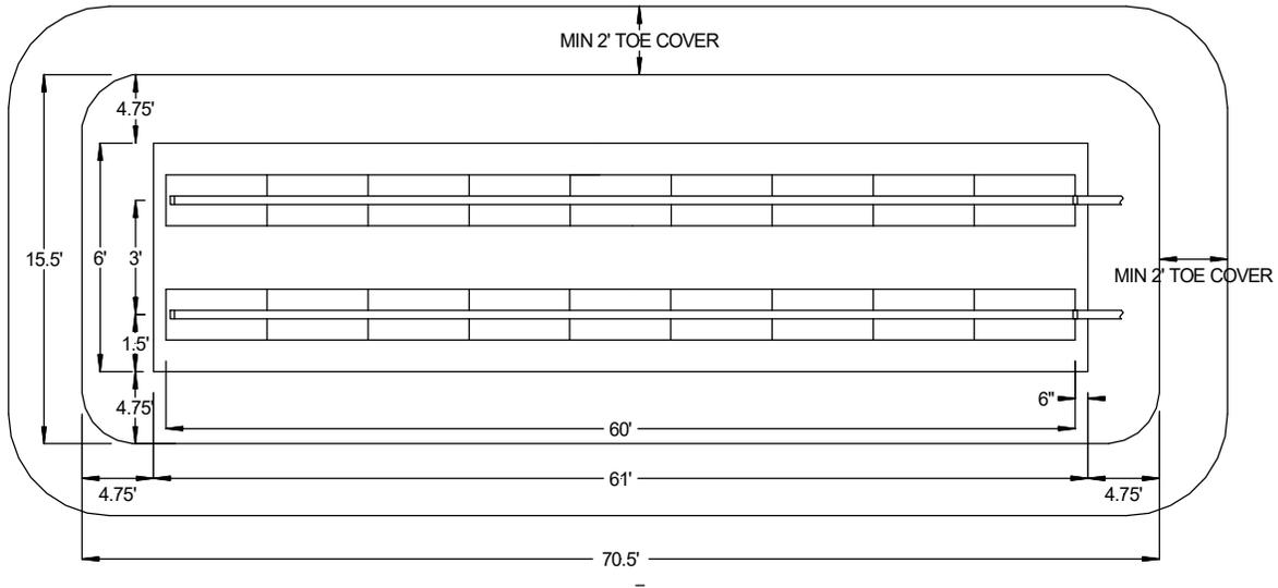
FIGURE 13: CROSS SECTION VIEW – BED SYSTEM – LEVEL SITE
