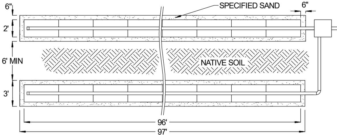
FIGURE 4: SECTION VIEW – TRENCH SYSTEM – LEVEL SITE
