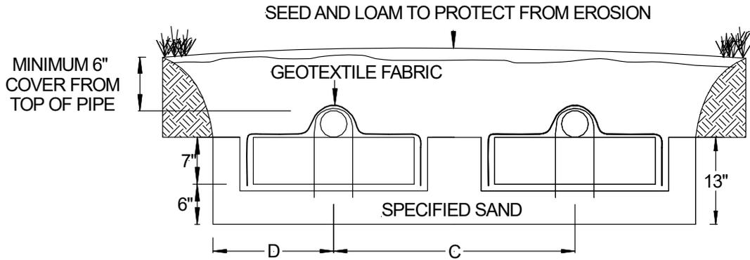
FIGURE 9: SECTION VIEW – 3 LATERAL BED SYSTEM
