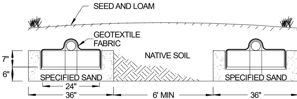
FIGURE 5: SECTION VIEW – TRENCH SYSTEM – SLOPING SITE
