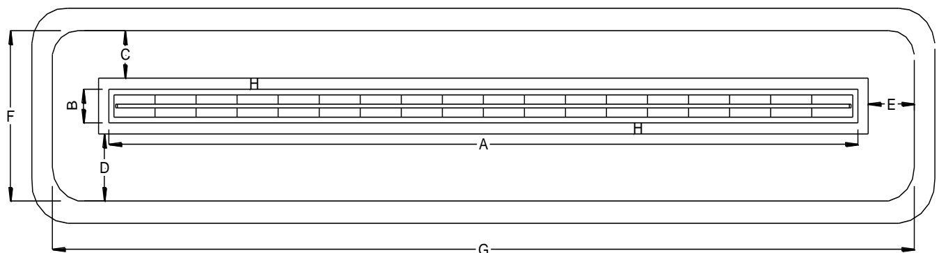
FIGURE 13: PLAN VIEW – MOUND SYSTEM
