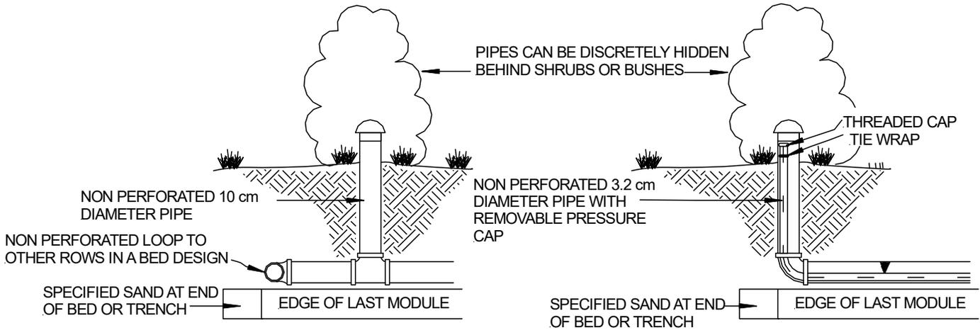
Figure 3: Air By-Pass Line Detail for Venting of Pumped Systems (when required)
