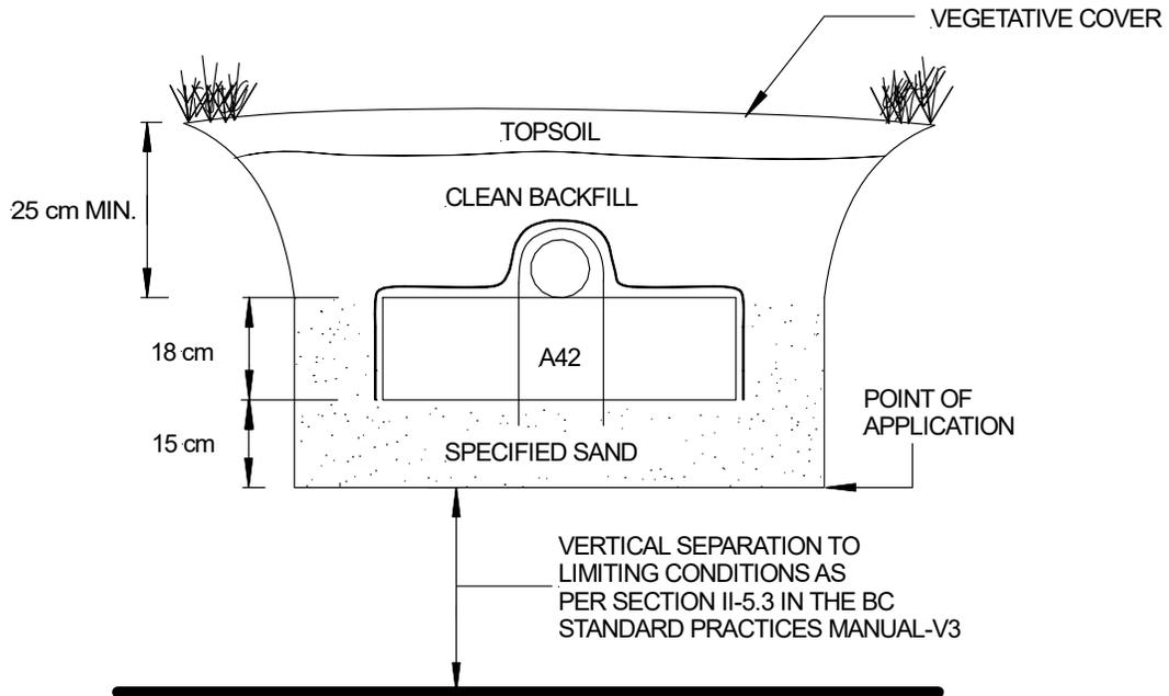
Figure 5: A42 Trench Cross Section
