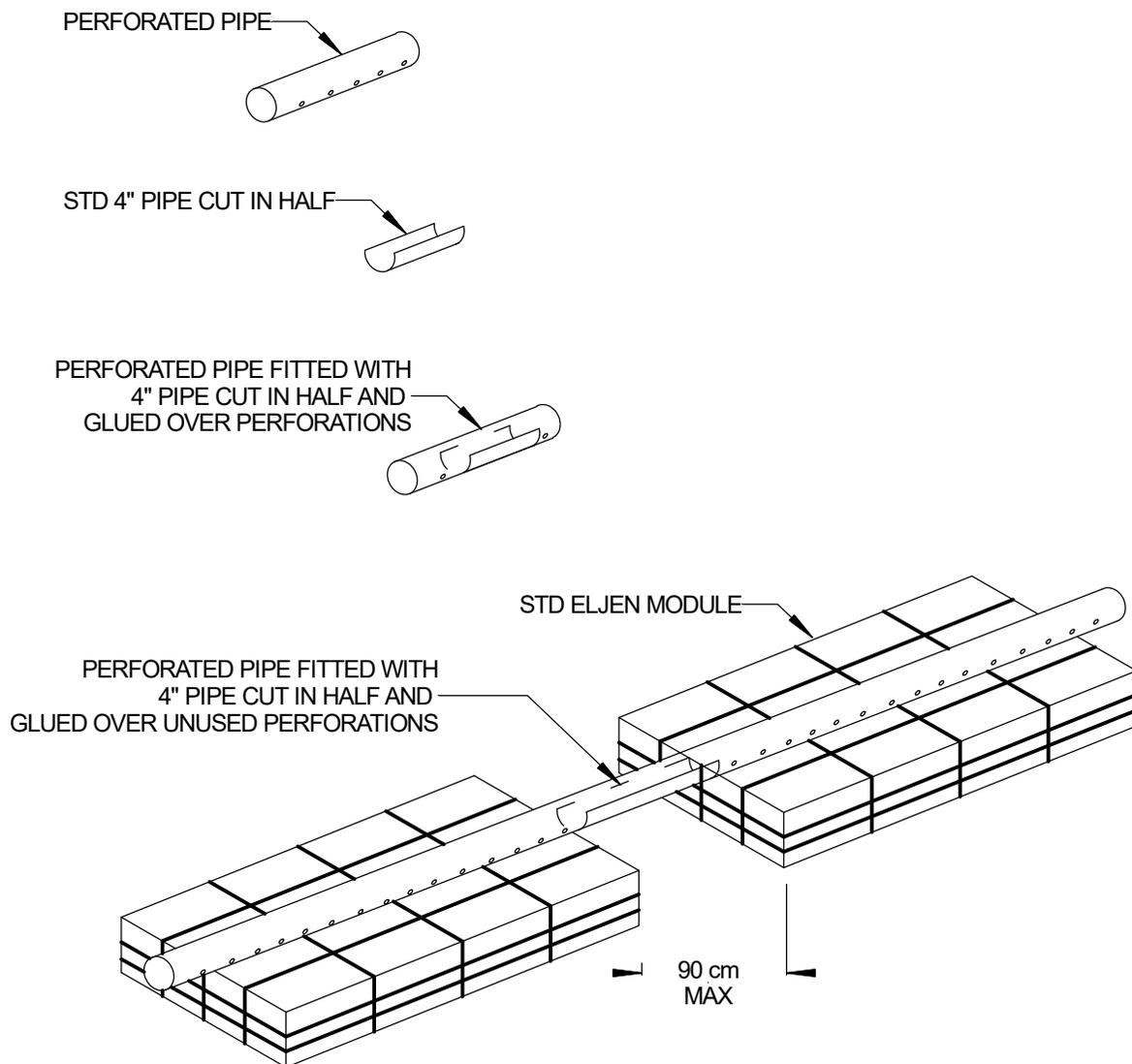
**NOTE:** Half-pipe must cover any hole above the A42 module that is within 15 cm of the edge. If modules are spaced end-to-end, fabric must be cut and allowed to drape over and protect the ends of each spaced module. A continuous run of geotextile fabric is not allowed for these applications.
