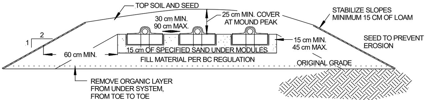
Figure 11: Raised Bed on Slope
